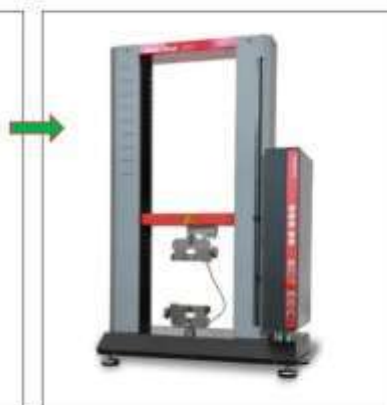
Picture 7: ProLine 2010 after modernization at ZwickRoell's premises
